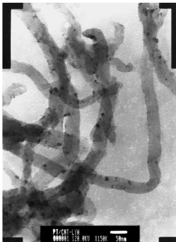
Fig. 2. TEM of the Pt/CNTs catalyst.
